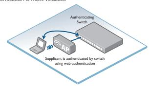
In a wired environment, where simple Extensible Authentication Protocol (EAP) pass-through switches are used at the edge of the network, then 802.IX or web authentication is performed on the authentication-capable switch at the aggregation layer.
