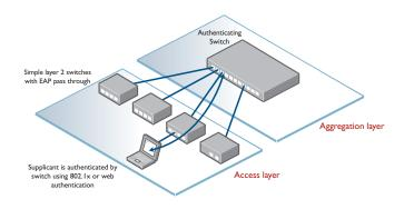
In this case, roaming authentication for dot1x or web authentication enables a user to unplug from one edge switch and plug into another without needing to re-authenticate. Roaming authentication can support the case that the user is connected directly to the authenticating switch.
